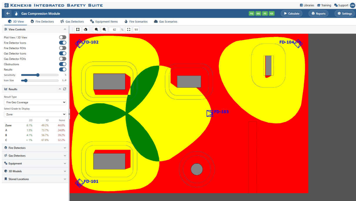
Figure 4-1. The plot view showing a fire geographic coverage result. Detector icons and name labels are drawn over the coverage map; the thin outlines around equipment are the graded-area boundaries; the toolbar provides area drawing, erase, zoom, Fit to View, and Actual Size.
