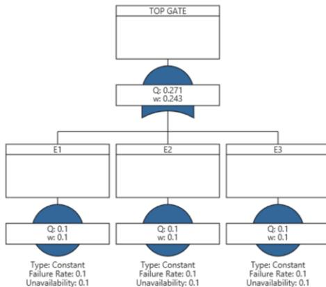
In this tree, there are three events E1, E2 and E3. The top gate is an OR gate, meaning that a failure of any one of the three events will result in failure of the top gate. For this simple fault tree, there are seven cut sets as follows:
