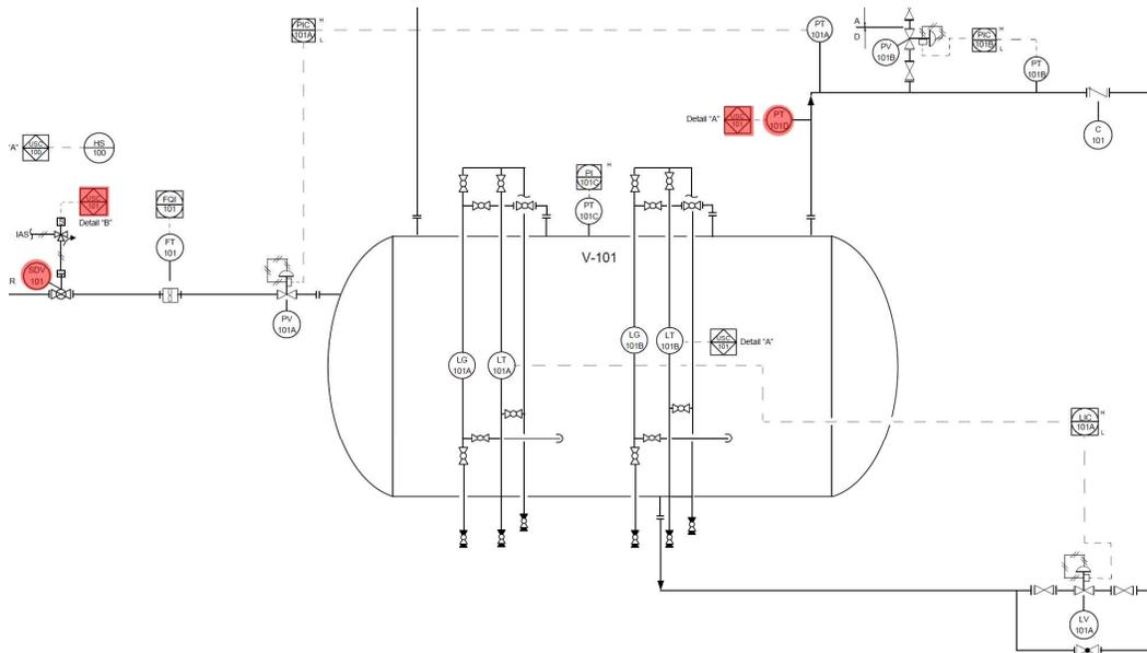
The SIF we'll be modeling is High-High pressure in V-101 (measured by PT-101D) causing closure of the input shutoff valve (SDV-101). This action is taken through interlock USC-101, which is a SIL 3 certified SIS logic solver.
