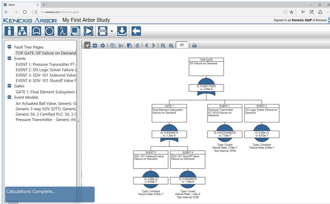
At this point our analysis is complete. We have calculated a top gate unavailability of  $9.1E-03$ . The unavailability of our top gate is another way of describing the  $PFD_{avg}$  for a Safety Instrumented Function. In this case our SIF has achieved a risk reduction factor (RRF) or 109, which is 1 divided by the  $PFD_{avg}$ .
