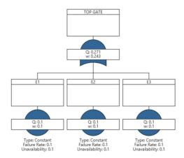
In this tree, there are three events E1, E2 and E3. The top gate is an or gate, meaning that failure of any one of the three events will result in failure of the top gate. For this simple fault tree, there are seven cut sets as follows:
