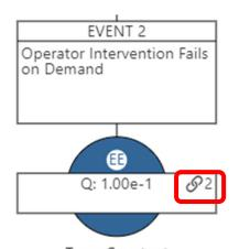
Type: Constant Failure Rate: 1.00e-1 Unavailability: 1.00e-1
