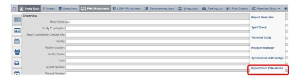
When Importing from PHA-Works, the data in the Open PHA study will be over-written completely. For this reason, it is usually the case that you will want to create a new Open PHA study in Open PHA Premium to receive the import.
