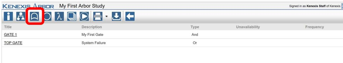
For large fault tree's it can be useful to display all gates in the tabular interface of the gates grid which allows for quick comparison of Unavailability or Frequency results between gates. From the Gates Grid View, the properties of a gate can be displayed by either double-clicking on a row of the grid, or clicking on the gate title.
