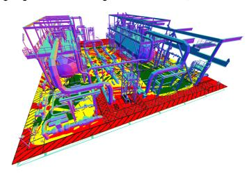
mapping software. This combination provides the most rigorous analysis, which results in the safest plant at the lowest cost by optimizing detector placement.
