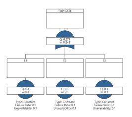
In this tree, there are three events E1, E2 and E3. The top gate is an or gate, meaning that failure of any one of the three events will result in failure of the top gate. For this simple fault tree, there are seven cut sets as follows:
